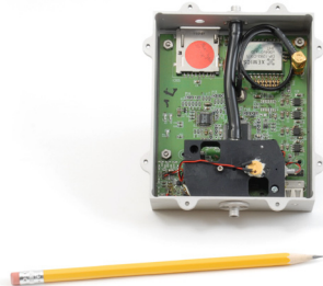
The miniPCS probe includes all the necessary electronics for remote operation and data acquisition.
