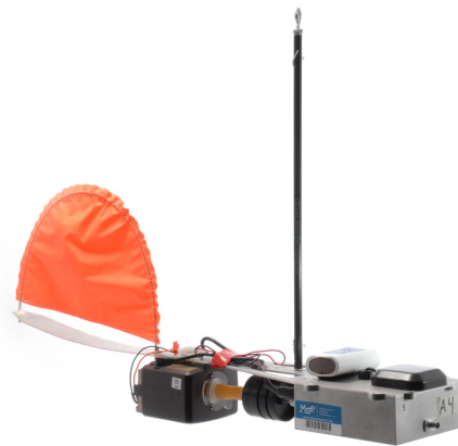
The miniPCS in field configuration. The air containing particles is pulled through the probe volume by the pump at the rear. A removable filter ahead of the pump is used collect particle samples.
