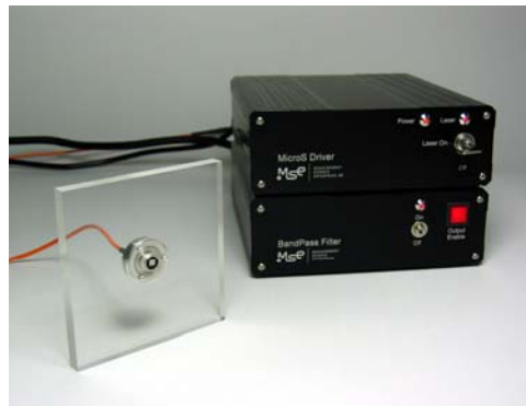
The microS system includes a microS probe, driver electronics, band-pass filter, and BP-microS acquisition hardware and processing software (computer is optional).
